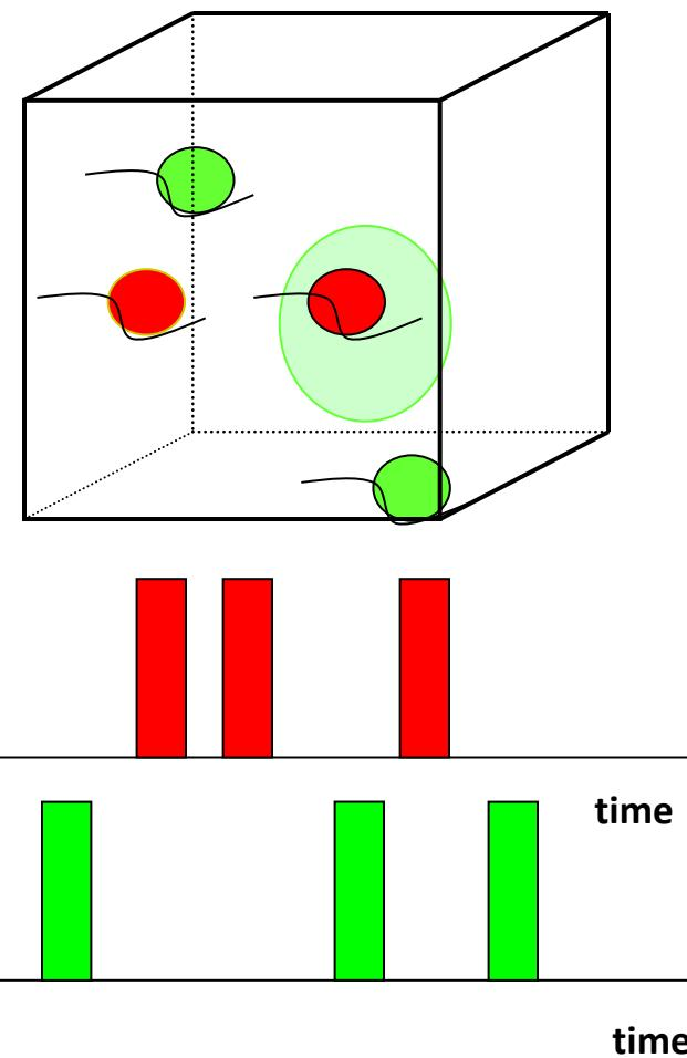
$$B_{CC} = \frac{\sigma_G \times \sigma_R}{\langle F \rangle_G \times \langle F \rangle_R}$$
