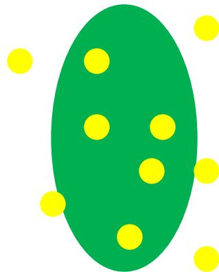
Fluorescent molecules diffusing into and out of the excitation volume cause fluctuations in the intensity that obey Poisson statistics
